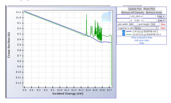
Looking at the plot of the absorption of  ${}^{1}H$  compared to  ${}^{27}Al$ , we can see the aluminum will absorb a lot more fresh, high-energy neutrons. As a result,  $k_{eff}$  is going to decrease.
